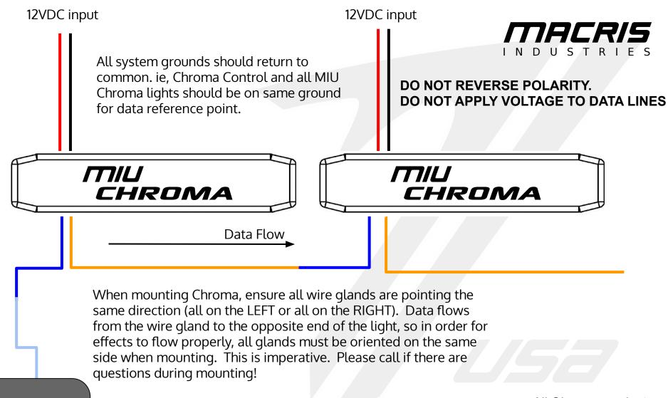
Control node has 3 wires: +12V (R) GND (B) Data Output (colored) Connect output wire of Chroma Control to Indigo input of MIU Chroma #1. Continue connecting output (orange) to input (indigo) until you reach the final light. The final output can be capped and bundled neatly and should not be connected to anything.
